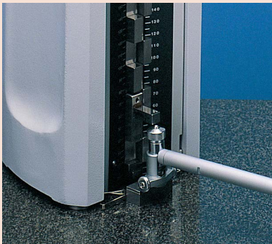
Bore gage zero-setting
